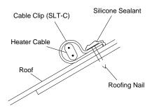
**Asphalt/Shake Shingle Roof** - Fasten with nail, coat nail head and upslope edge of clip with silicone sealant.
